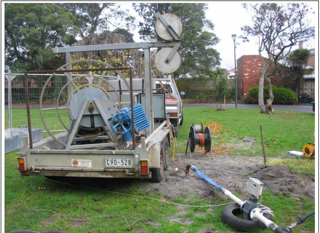
**Pumping test trailer established over borehole**
